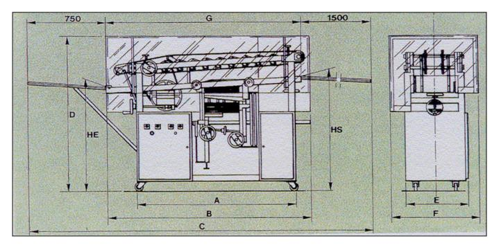
A : 1750mm F : 850mm Net weight: 400 kg B : 2240mm C : 4320mm G : 2050mm HE : 1060mm Brut weight: 600 kg D : 1540mm E : 655mm HS : 1100mm Shipping size: 2.44x1.12x1.85 m
