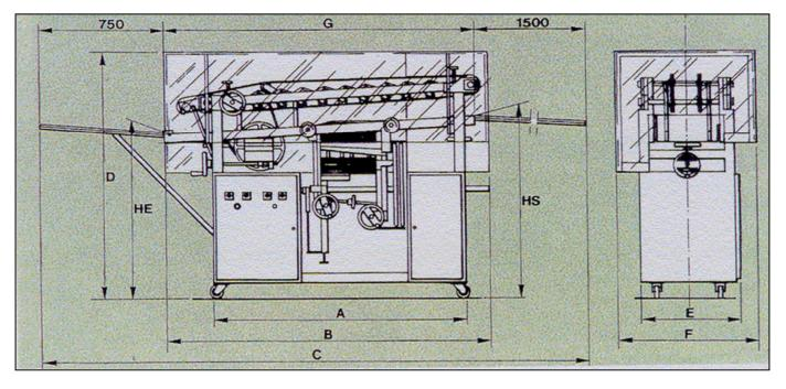
A : 1410mm F : 850mm Net weight: 400 kg B : 1840mm G : 1665mm Brut weight: 530 kg
