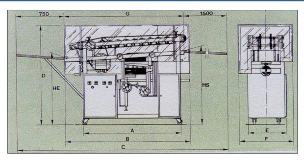
A: 1410mm B: 1840mm C: 3915mm D: 1500mm E: 655mm F: 850mm G: 1665mm HE: 1000mm HS: 1040mm
