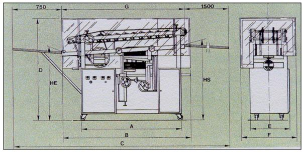
A : 1410mm F : 850mm Net weight: 380 kg B : 1840mm G : 1665mm Brut weight: 530 kg C : 3915mm HE : 1000mm D : 1500mm E : 655mm HS : 1040mm Shipping size: 2.08x1.12x1.66 m
